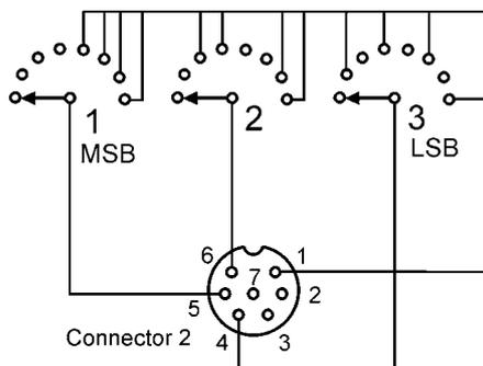
Figure 7 : Rotary switch connections
