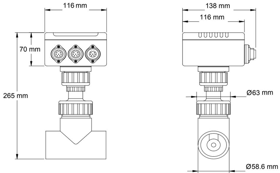
Figure 2 Head-mounting component dimensions
