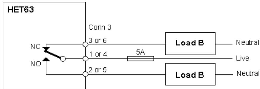
Figure 5 : Relay contact connection
