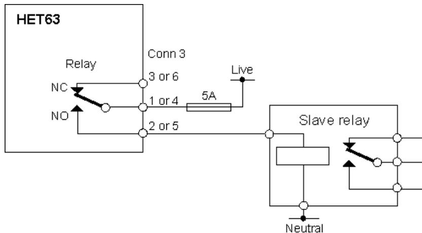
Figure 6 : Slave relay connection
