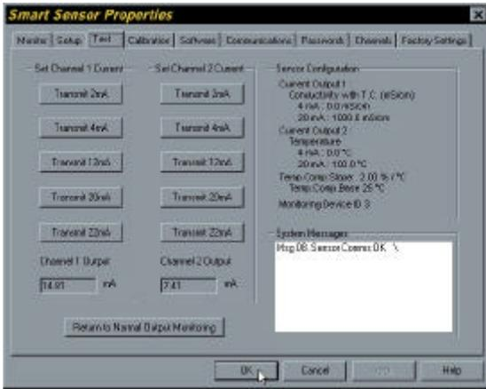
The Test Tab gives the user a series of buttons which force the sensor current outputs to fixed levels of 2mA, 4mA, 12mA, 20mA, or 22mA for each of the two channels. Both are independent and can be set the same or different in this mode.
