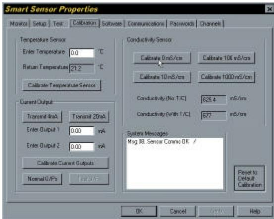
The three main calibration operations are grouped together on this Tab.
