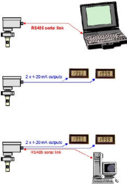
Configure, test, calibrate and monitor IET40 using the custom designed Smart Control Centre Windows 95 application software. The software is supplied on CD-ROM or is downloadable from [www.lth.co.uk](http://www.lth.co.uk)
