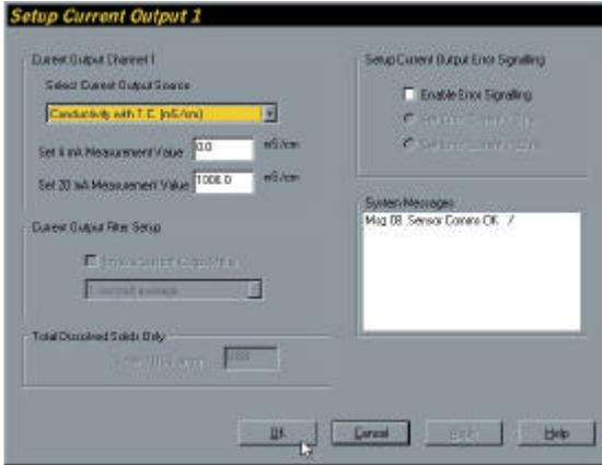
To Setup the Channel One Current Output, first select an Operating Range or Source from the List Box. Then set the 4 mA and 20 mA values from within the selected range.
