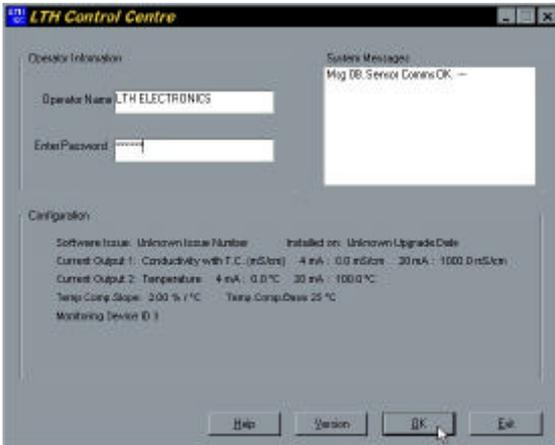
The LTH Smart Sensor Interface is a new way of configuring your instrumentation. The programme has been designed to maximise control over every aspect of the sensor's performance, from software loading and upgrading, to configuring and commissioning, through to monitoring the output of information from the sensor.
