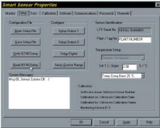
The Sensor Setup Tab is the lead in screen for configuring the majority of the IET40 options.
