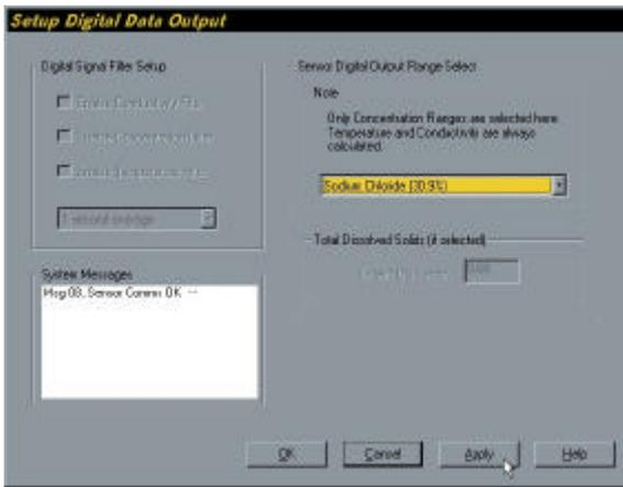
To Setup the Digital Data Output, first select an Concentration Range if required from the List Box. It can be disabled by selecting Concentration Not Required.
