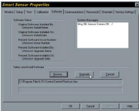
The upgrade files required to carry out a software update will be available on the LTH Web site, and will be free to download. Also on floppy disk (at a pinch) the updated files are simply copied into the “\Program Files\LTH Smart” folder and the Smart Sensor Programme is executed as normal.
