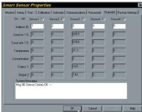
This Tab consists of 5 Groups of Instrument Monitoring Windows. It allows the operator to view up to 5 Sensors at the same time. No programming or modifications can take place in this mode. It is only active when this page is being displayed by the application. The Computer interrogates each Sensor in sequence and its data boxes are updated. Six Data measurements are extracted
