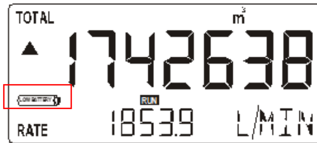
Fig. 4: Example of low-battery alarm.
