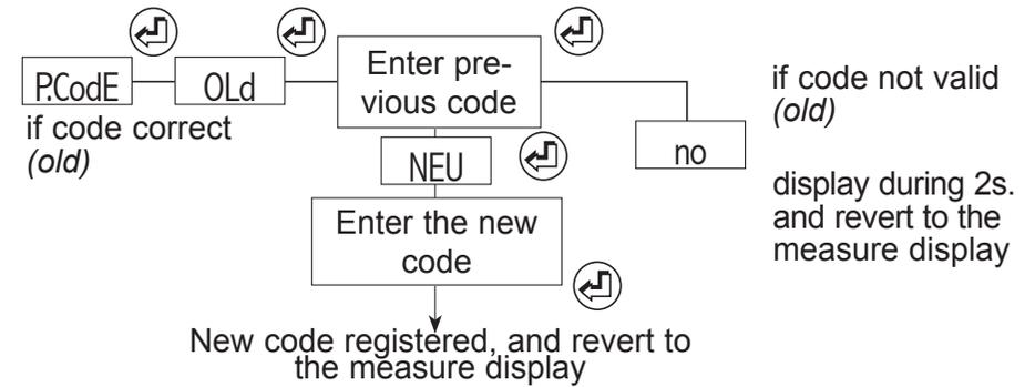
**Reminder:** If no key is pressed during 1 min, the instrument will revert to the measure display. On factory exit, the access code is 0000.
