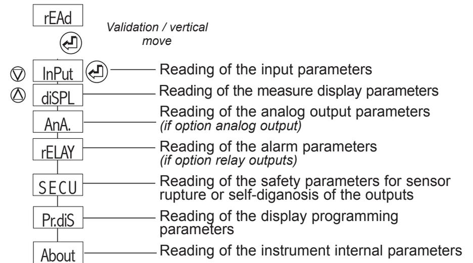
In each reading submenu, use keys  and  to move, and key  to visualise the parameters.
