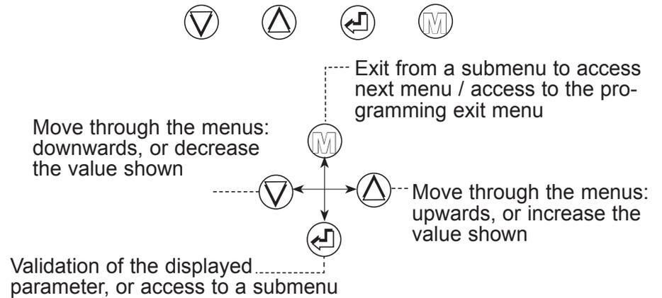
**Note:** In mode programming, the instrument will automatically revert to the measure with the former configuration if no key is pressed during 1min.
