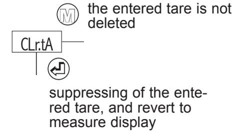
**Reminder:** If no key is pressed during 20 s., the instrument will revert to the measure display.
