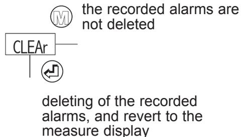
**Reminder:** If no key is pressed during 20 s., the instrument will revert to the measure display.
