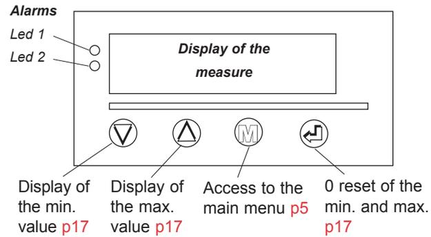
Further functions can be accessed by pressing several keys simultaneously:
