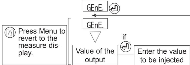
**Note:** The instrument will carry on measuring during the simulation. Only the analog output will no longer react to the measure.
