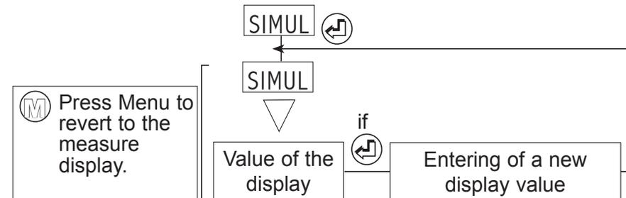
**Note:** The instrument will no longer measure during the simulation. The analog output and the relay outputs will react according to the entered display. If alarm messages have been programmed, they may appear during the simulation.
